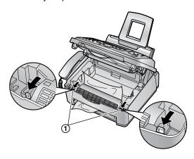
3. Remove the jammed paper (①) from the fuser unit by pulling it upwards carefully, then install the drum and toner unit.
